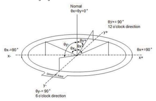
Figure 2 Definition of Viewing Angle
