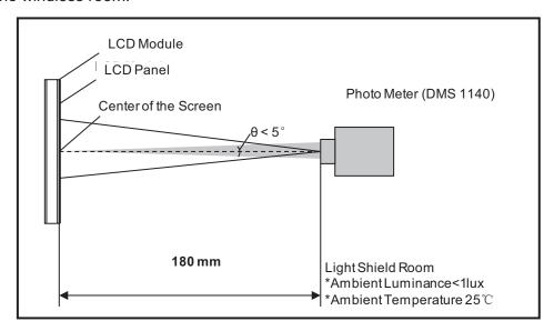
Figure 1 Optical Characteristic Measurement Equipment and Method
