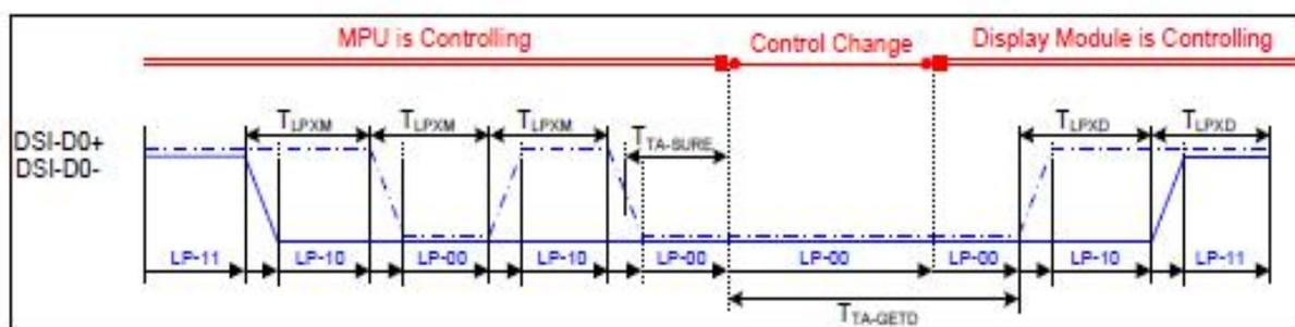
Bus Turnaround (BTA) from MPU to display module Timing
