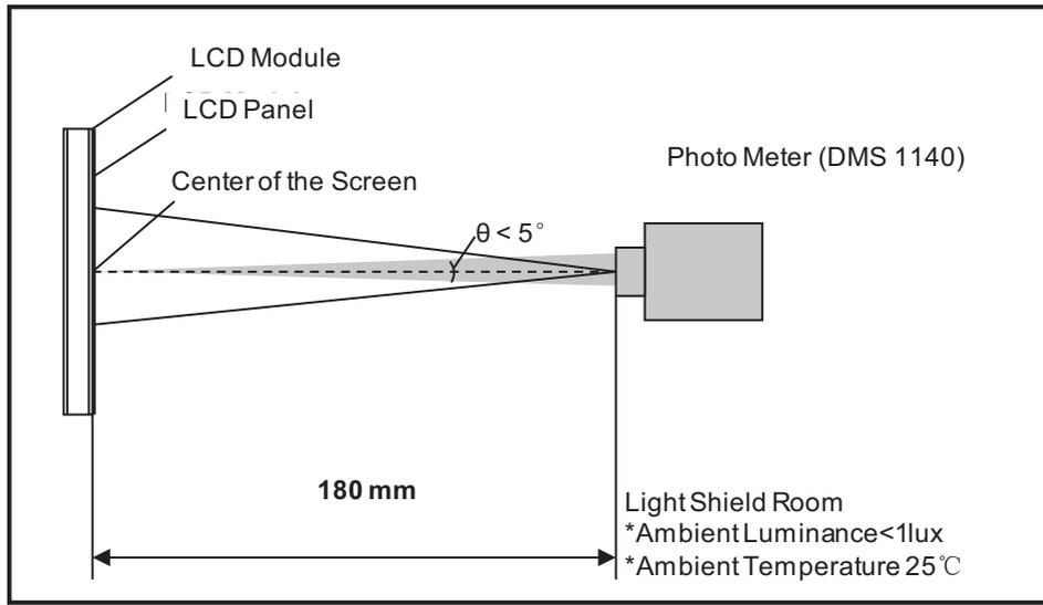
Figure 1 Optical Characteristic Measurement Equipment and Method
