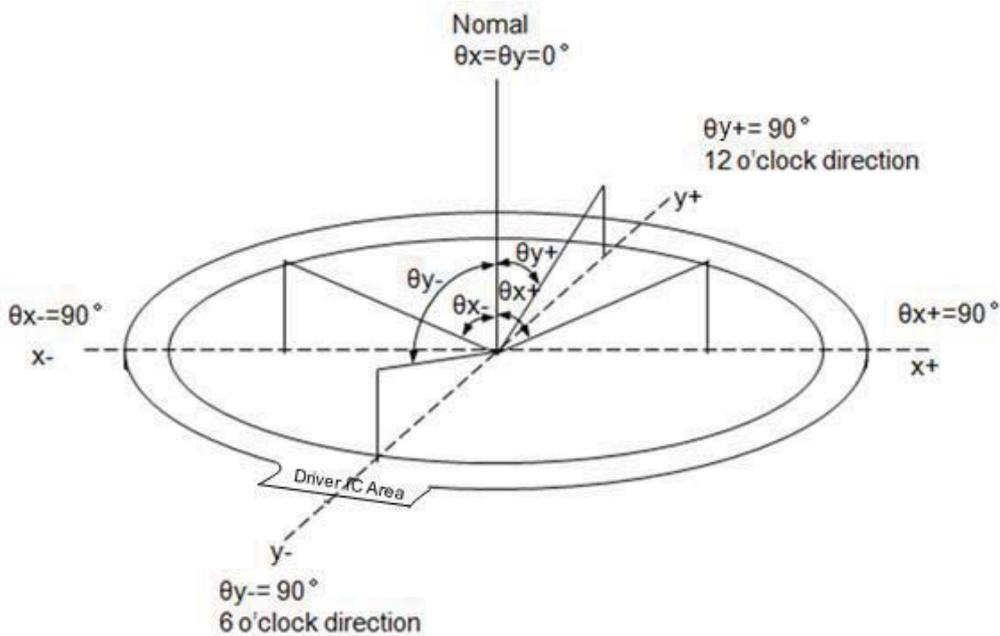
Figure 2 Definition of Viewing Angle
